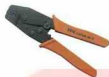
强力压著端子钳 YAC-5 适当管形端子 0.5-0.75mm 2 22-20AWG 1.0-1.5mm 2 18-16AWG 2.5mm 2 16-14AWG 4mm 2 14-12AWG 8mm 2 12-10AWG
